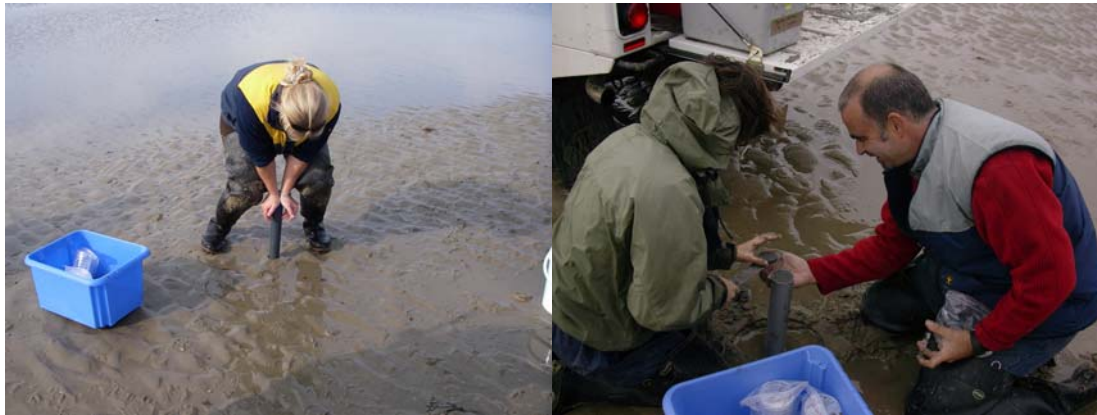
Figure 5 : Manipulation of the corer (left) and slicing the sediment (right)
